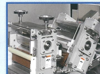
■ Sub Dough roller (Double Pressing function)
