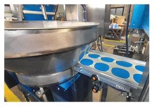
Fresh dough and off-cuts are evenly blended by the twin screw mechanism to produce a consistent dough sheet, which is then fed into the attached gyoza machine.
